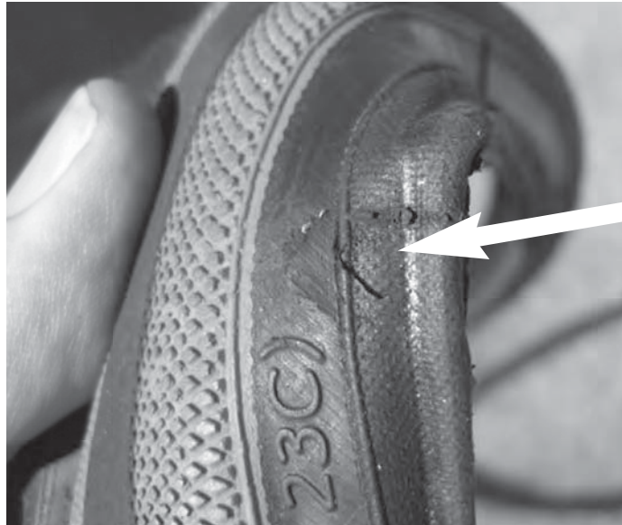
The arrow shows where the tire has been cut and now requires a boot.
