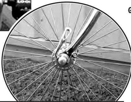
Radially-laced front wheel is replaced with a Schmidt hub on longer brevets.
