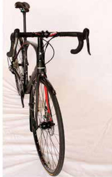
Alans Carbon Liscio II with SRAM Red22, fenders, and SD-8 generator Hub. Our solution for the lightweight brevet machine.
